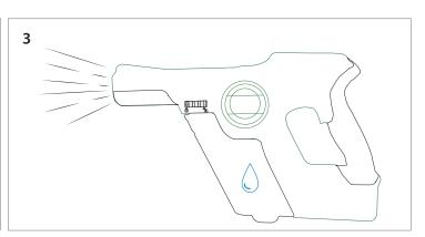
To reduce the chance of blockage we recommend that after every few days of use spray a tank of water through the unit to rinse out any residual chemical build up that may have occurred.
