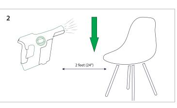
Start spray application on the highest point of the surface on the object being disinfected and quickly move to the lower areas. Where possible, sprayer should be kept as level as possible and be approximately 2 feet (24") from the surface being treated.
