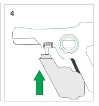
Re-attach the tank by aligning the vertical rails of the sprayer with the groove along the top of the tank. Rotate the collar lock to the "lock" icon.
