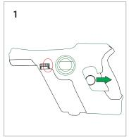
To remove the solution tank from your Victory Sprayer, simply rotate the collar lock to the "unlock" icon and pull the ring back to release the locking mechanism.
