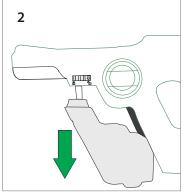
You can now pull the tank off the Fill the tank with the desired unit.
