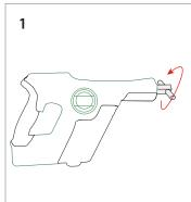
To clean or unclog the nozzle, remove the nozzle using the nozzle wrench provided and rotating it in counter-clockwise direction.
