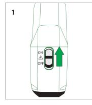
Push the electrostatic charge switch to the "On" position.
