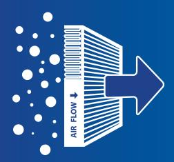
HEPA stands for High-Efficiency Particulate Air. HEPA media filters are most commonly known for their use in vacuum cleaners. The HEPA media filter is designed to remove small particulate or floating matter from the air and trap it inside the cleaning appliance.
