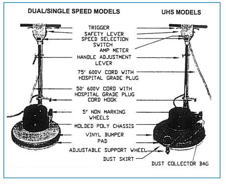
bottom). The drive pad must seat fully. Center the floor pad and press lightly to allow the drive pad to grip it. Uhs models: Drive pad and floor pads are already installed before shipping. The floor pad may be replaced by turning the "Center-Lok" counter clockwise to remove. Replace pad by centering it on drive pad and re-install "Center-Lok".
