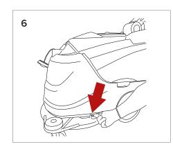
Turn valve manually to adjust water level.
