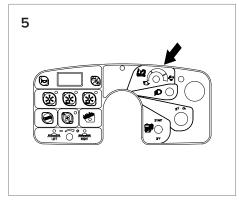
Toggle switch to change drive direction to Forward or Reverse.
