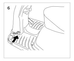
Press accelerator pedal to activate drive.
