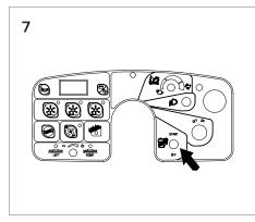
Press and hold for +3 sec. to manually activate filter shaker.
